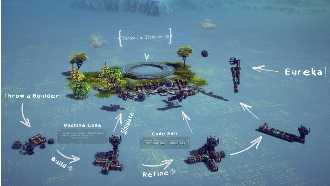
Figure 1: The task of compositional machine design is illustrated in our BesiegeField environment. The figure shows a high-level sketch of the agentic workflow (w/ Gemini Pro 2.5), along with the resulting machines and their simulated performance. The design objective is to create a machine that throws boulders long distances.
